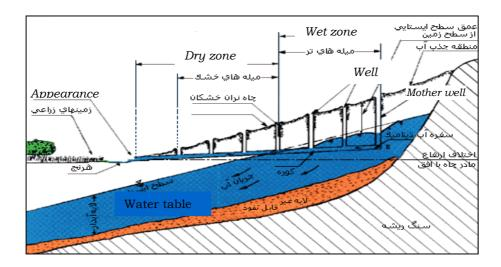
Figure 1- Characteristics and building terms of qanat (Nasseri, 2005).
