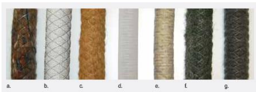
Figure 3. Envelopes can be made of wrapped polypropylene fibres (a, f & g), polystyrene granules (b) and coconut fibres (c), non-woven nylon (d) and woven typer (e)
