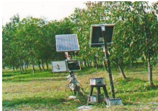
Figure 6 - Measurement of transpiration rate with sap-flow meter. Source: Jeet Ram et al., 2008
