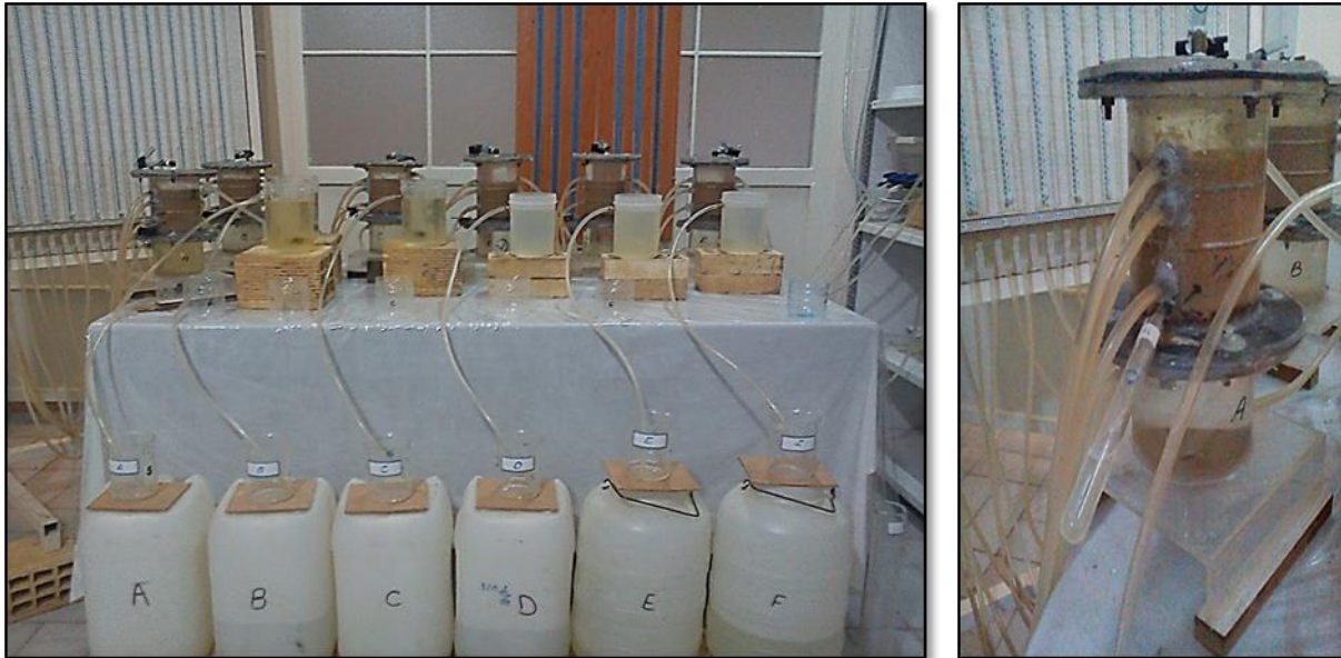
Figure 2. Sampling the drainage water extracted from the apparatus
