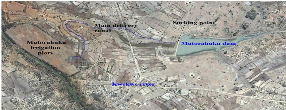
Figure 4. Mutorahuku irrigation scheme-showing the gravity powered system from the dam to the irrigation plots
