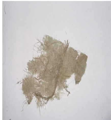
Picture 1. PFM penetrated by roots
