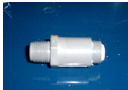
Figure 7. Emitter is ready to be connected using pipe
