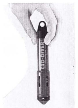
Figure 11. Compact data logger diver for measurement groundwater level, temperature, PH, and conductivity
