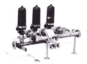
**Figure 14b.** An automated filtration set consist of controller, hydraulic valves, self cleaning and automatic backwash helix disc filters, manometer, air relieve valve
