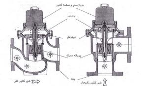
**Figure 17.** Metering valve in two types, vertical (left), angled (right)
