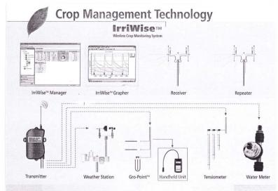
Figure 10. Components of a wireless crop monitoring system
