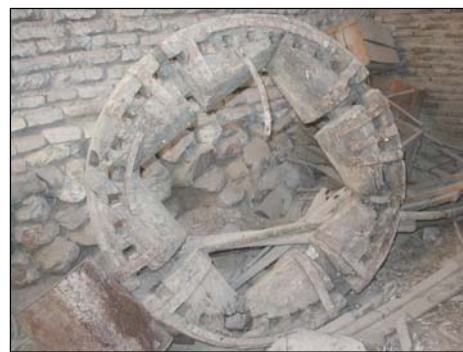
Gears of water wheel
