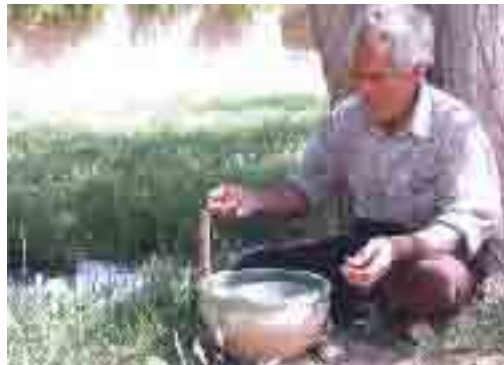
Figure 2- calculating water shares by means of a traditional clepsydra
