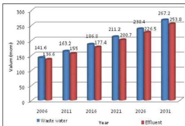
Fig. 7. Estimation of wastewater and effluent production of Mashhad metropolitan city (million m<sup>3</sup>/y)
