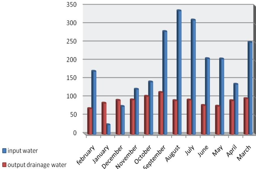
Fig. 1. Monthly volume comparison of input water with output drainage water from Dez basin networks (2010 - 2011)
